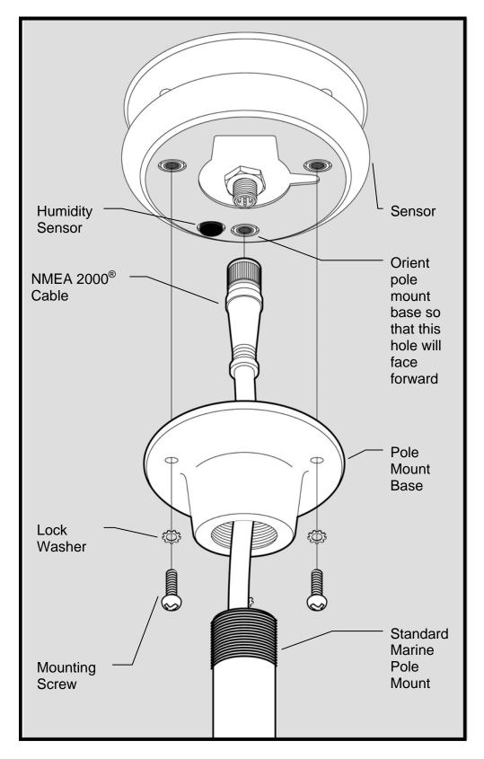
Figure 1 – Mounting the WSO100 to a Standard Marine Pole Mount
