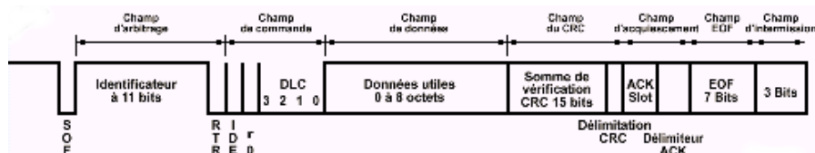
FIG. 1 – Trame CAN standard
